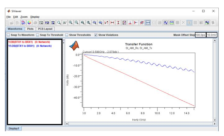
To add a new display, right-click on the display name tab and select **Add New Display**. Select the **Show Pulse Response (Unequalized)** and view it.
