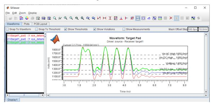
Similarly, to view the effect of changing the transmission line length, select the rows corresponding to 50 ohm resistance and 2 in, 4 in, 6 in, 8 in, and 10 in length.
