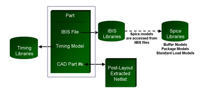
A Part has a unique identifier and contains references to an IBIS file, a timing model, and a CAD part number. An IBIS file, in turn, may contain:
